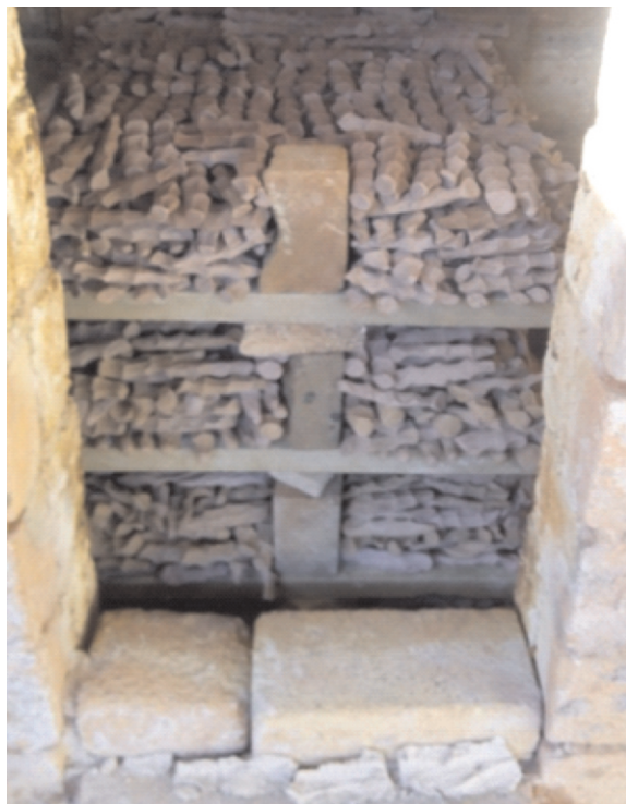
Figure 8:carefully arranged on shelves in the kiln for firing
