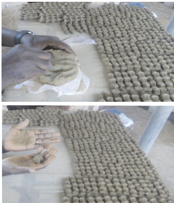
Figure 1: pinching the plastic clay
